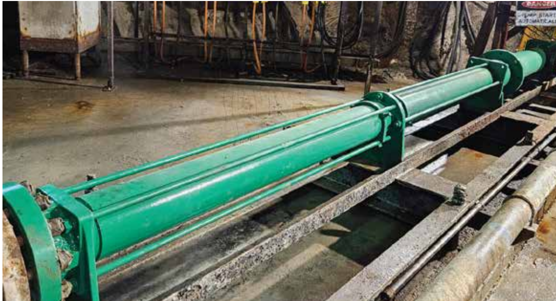
Roto Flex Pump Handling Hyper Saline Mine Water with Suspended Solids
