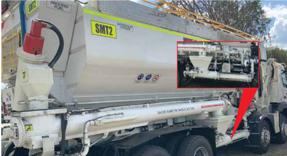
Mobil Manufacturing Unit (MMU) with Mounted Pumps run via Hydraulic Motors
