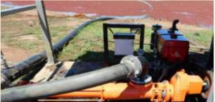
Package includes Pump, Drive, Clutch, Belt & Pulley Drive options are Diesel Engine, Petrol Engine or Electric Motor
