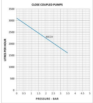
Tested on water at 20° and 1450 rpm
