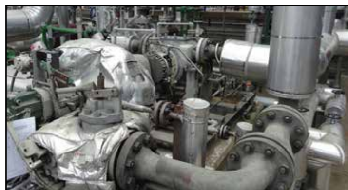
Vacuum Residue at Refinery - Ecuador Flow - 48 m 3 /hr, Pressure - 11 bar
